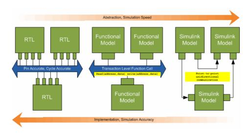
The functional model provides a sort of halfway point between the speed you can achieve with abstraction and the accuracy you get with implementation.
