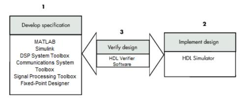
As the figure shows, HDL Verifier software connects tools that traditionally have been used discretely to perform specific steps in the design process. By connecting these tools, the link simplifies verification by allowing you to cosimulate the implementation and original specification directly. This cosimulation results in significant time savings and the elimination of errors inherent to manual comparison and inspection.
